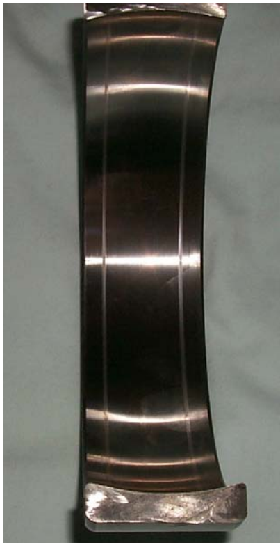
Figure 10. SKF 2218 Outer Ring Damage.
