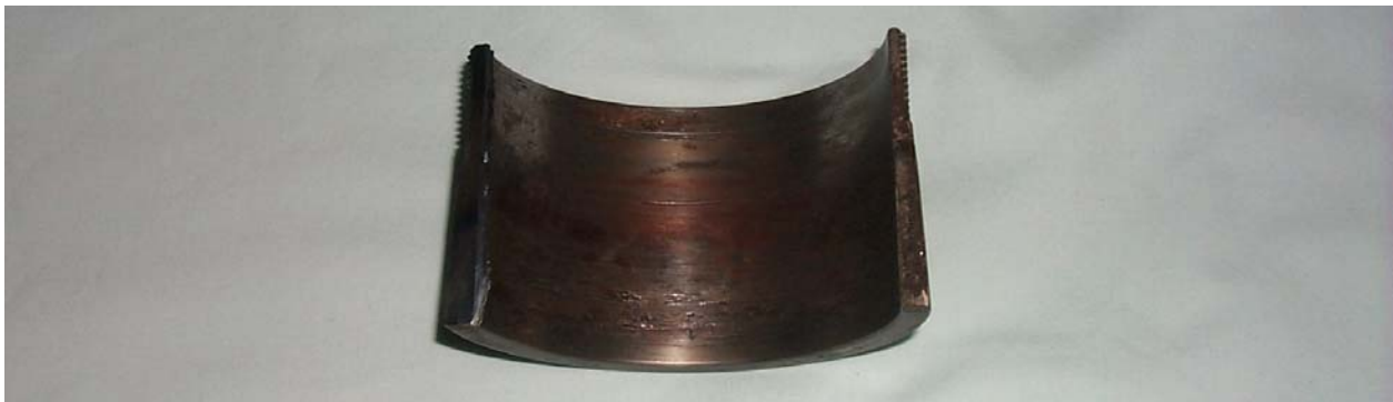
Figure 13. Fretting Corrosion on Taper Lock.
