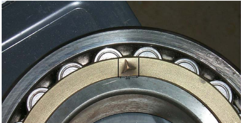
Figure 2. Damaged Cage, SKF 22222.
