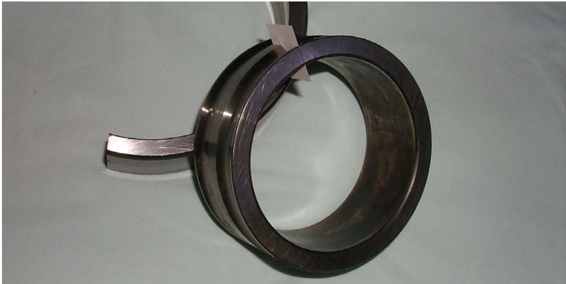
Figure 7. SKF 2222 With Cracked Inner Ring.
